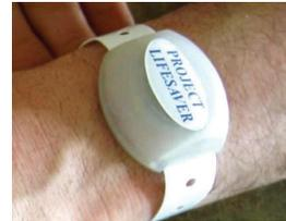
The bracelet is much more than an ID bracelet. It is a one ounce battery operated radio wrist/ankle transmitter emitting an automatic tracking signal every second, 24 hours a day. Each bracelet has a unique radio frequency allowing the search team to positively locate and identify the person that has wandered away from home or a care facility. The signal is tracked on the ground or in the air.
